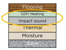
The conventional floor construction, including the underfloor heating, has a thickness of 92mm. The heating elements alone are 62mm thick and consist of a variety of components
